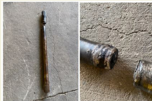
Figure 4. Damaged axle shaft
