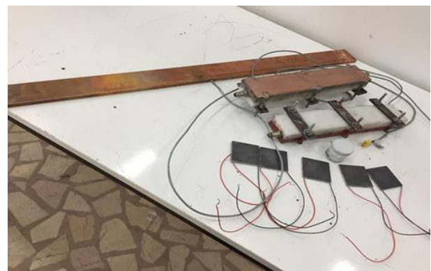
Figure 3. Copper receiver plate, heat sink and thermoelectric module
