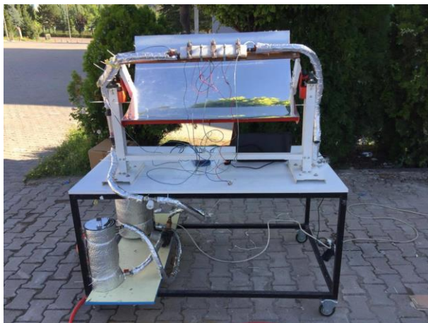
Figure 1. Setup view with piping system and storage tanks
