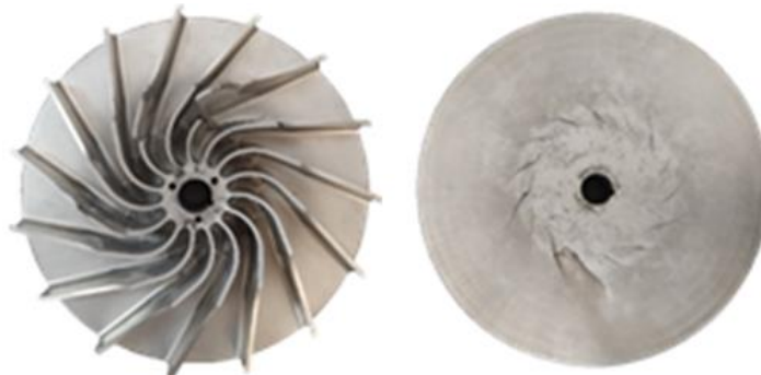
Figure1. Damaged Blower Impeller
