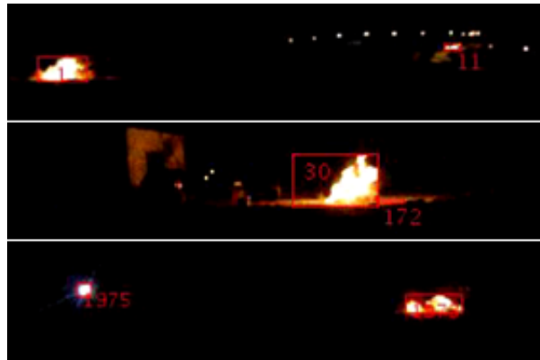
Figure 4. Examples of false detections are shown. TOP: The fire on the left (Object tag: #1) is correctly detected. However, flashlights of the cars passing by (Object tag: #11) are falsely labeled as fire object. MIDDLE: Fire (Object tag: #30) is correctly detected while its reflection (Object tag: #172) is also falsely detected, BOTTOM: (Object tag: #1975) is a correctly detected fire. (Object tag: #1873) is a flashlight and it is a false detection.
