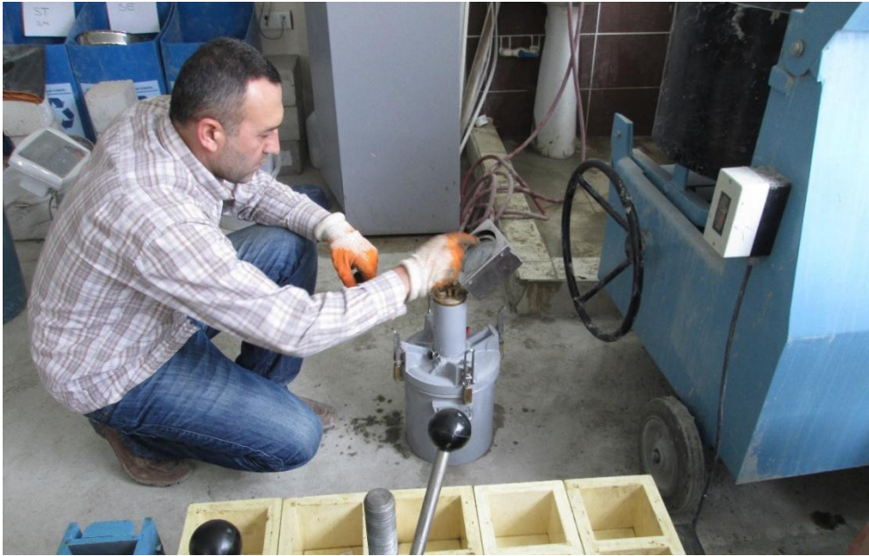
Figure 4. Measurement of the amount of air in fresh concrete
