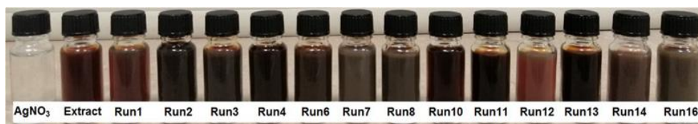
Fig 5 Changes in solution colors confirming the formation of AgNPs in different experimental runs
