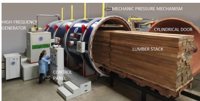
Fig. 2. General view of a high frequency - vacuum combination drying kiln with a capacity 25m 3 [3].
