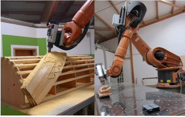
Figure 14. Manufacturing furniture through 7-axis robot [6]
