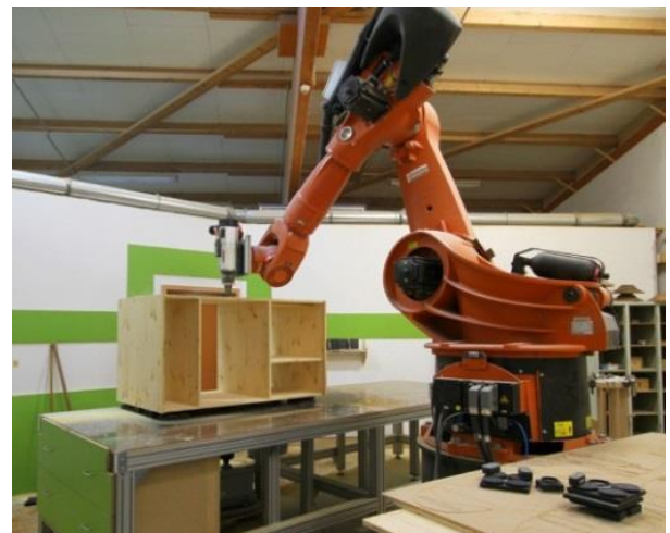
Figure 13. Manufacturing furniture through 7-axis robot [6]
