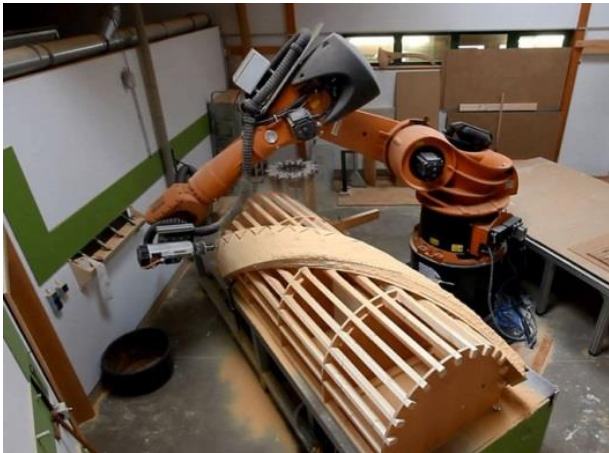
Figure 15. Manufacturing furniture through 7-axis robot [6]
