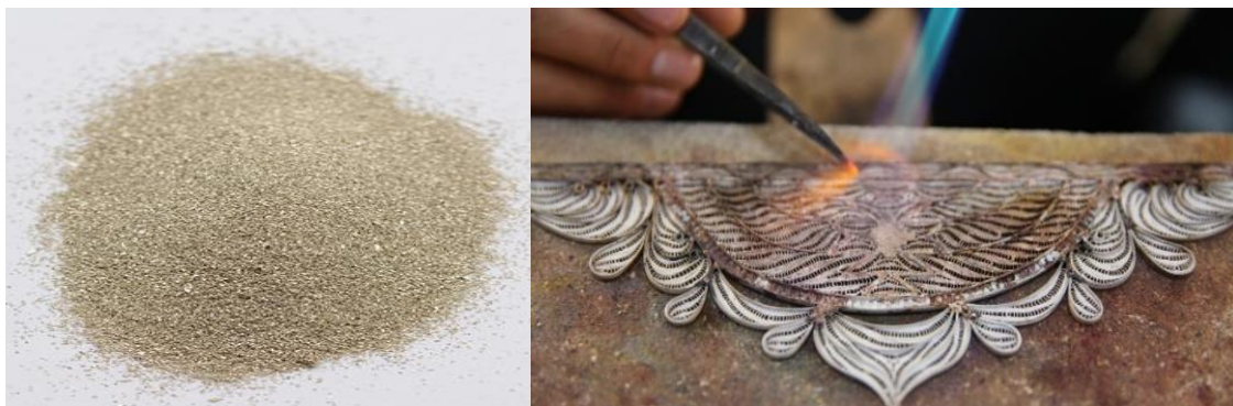
Figure 2. a) Jewelry welding powder, b) jewelry welding powder operation
