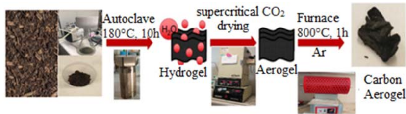
Figure A. Synthesis steps of carbon aerogel from biowaste
