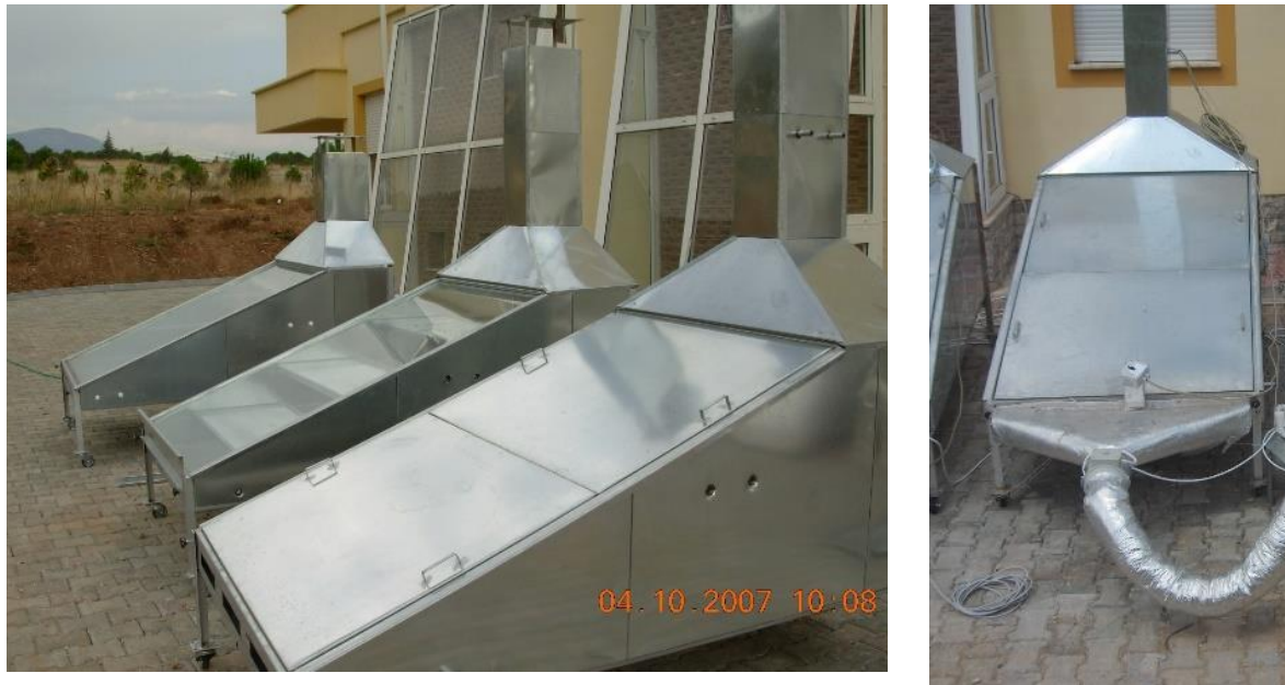
Figure 1: Ambient air drying, solar water collector assisted drying and solar air collector assisted drying cabin-type dryers used for experiments in the study.
