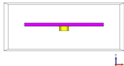
Figure 10.c. Antenna # 3 feed point side view
