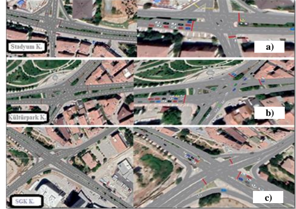
Şekil 8. Sola Dönüş Cebi Eklenmiş 2D/3D PTV Vissim Çizimleri (a) Stadyum Kavşağı, (b) Kültürpark Kavşağı, (c) SGK Kavşağı (2D/3D PTV Vissim Drawings with Special Left Turn Lanes (a) Stadium Intersection, (b) Kültürpark Intersection (c) SGK Intersection)
