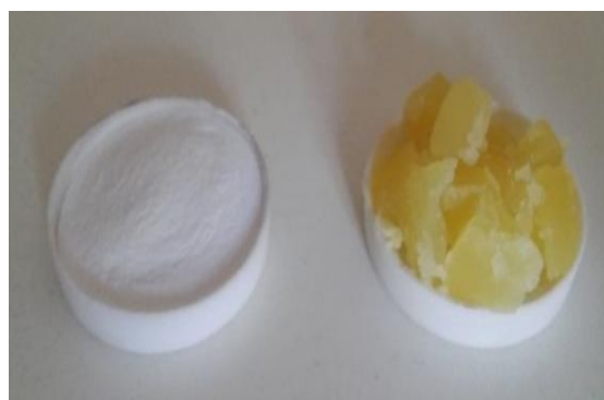
Figure 5. The magnesol absorbent before and after the purification process
