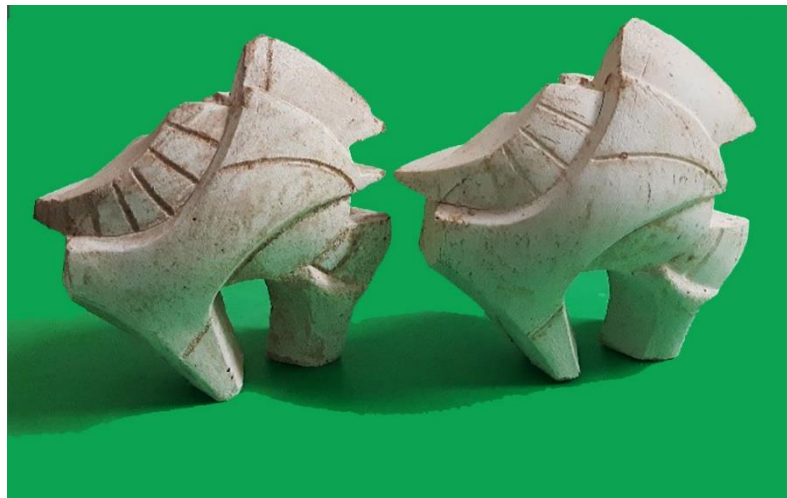
Figure 4. “Model A” form formed with AC mixture after heat treatment at 1200 oC (Filiz, 2022)
