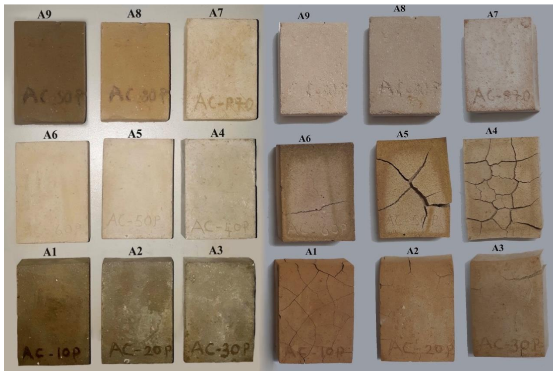
Figure 1. The image of all mixtures between A1 - A9 after shaping in a silicone mold (left), and after firing at 1200 °C (right) (Filiz, 2022)
