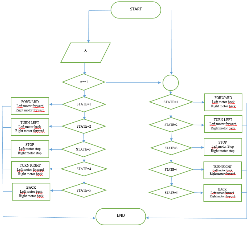
Fig. 9. Flowchart of Tank Robot Android Application
