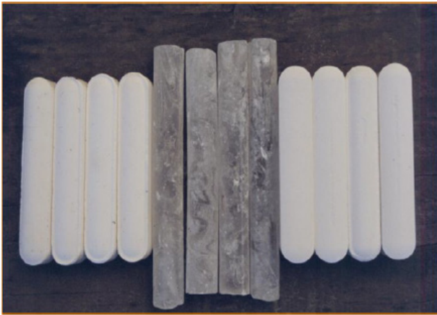
Figure 7. Examples of fused boron, boron/fluoride and a dazomet rod (left to right).
