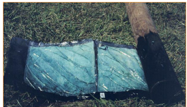
Figure 2. Example of a self-contained copper/boron preservative bandage
