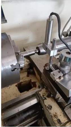
Figure 1. The clamping system of the lathe, workpiece and cutting tool
