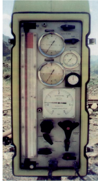
G TİPİ PRESİYOMETRE / G TYPE PRESSUREMETER
