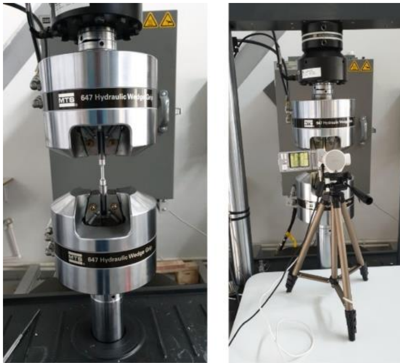
Figure 7. Fatigue testing of road wheel test specimens
