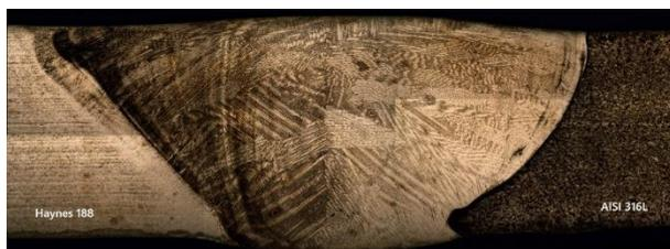
**Figure 6.** Haynes 188 - AISI 316L weldment macrostructure image.
