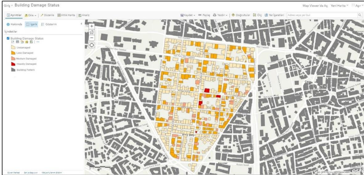
Figure 6. Post-Earthquake Damage to The Building Stock
