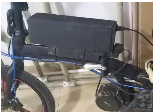
Fig. 12. Electric bike with battery pack and BMS
