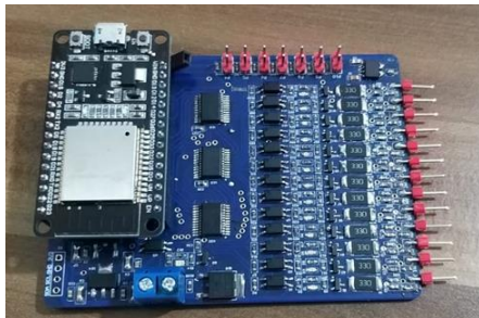
Fig. 8. Real time implemented designed BMS circuit
