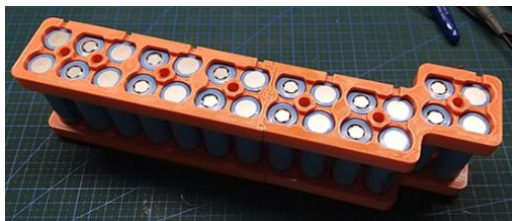
Fig. 9. Designed battery pack top view
