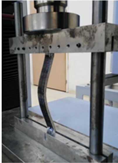
Figure 3. Deformation of the Hybrid Composite Sample After the Buckling Test
