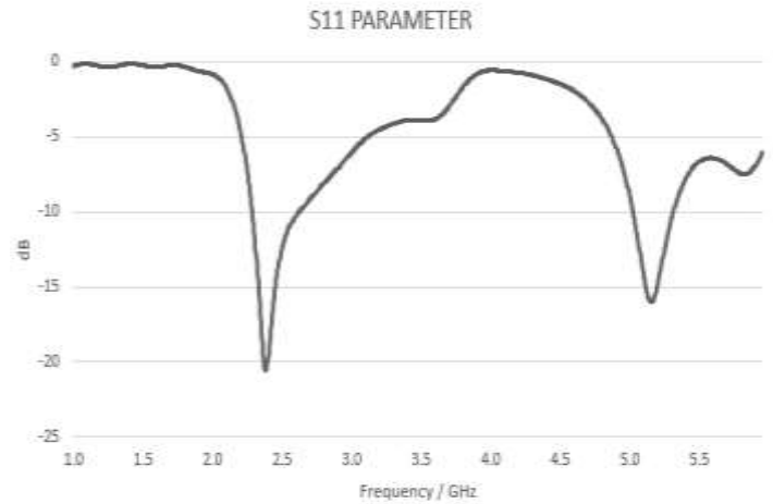
Fig. 3 S11 graph of proposed antenna
