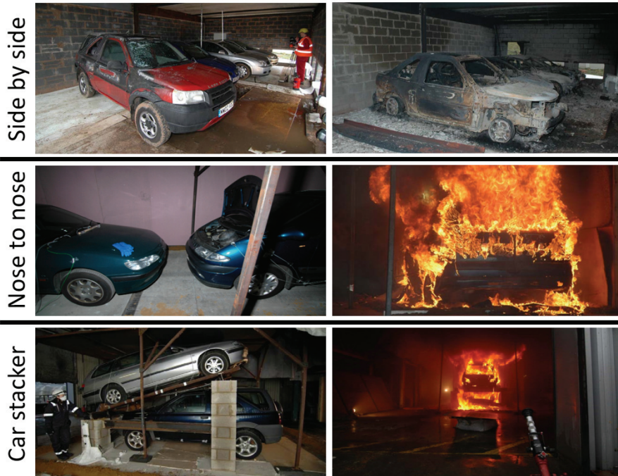
Fig. 3 - Fire spread between passenger cars (BRE,2010 [13]).
