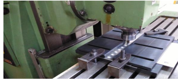
Figure 4. The milling machine used for friction stir spot welding process
