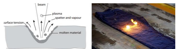
Figure 7. Laser Fading Process in Denim Fabrics [91]
