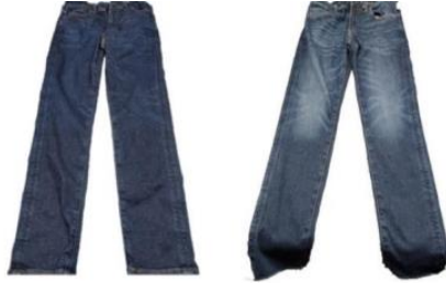
Figure 6. Before and After Ozone washing in denim [88]
