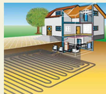
Figure 1. Schematic drawing of ground source heat pump system
