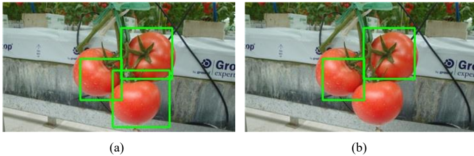
FIGURE 5. An example of the classification of HOG and LBP features by (a) SVM and (b) kNN for tomato detection.
