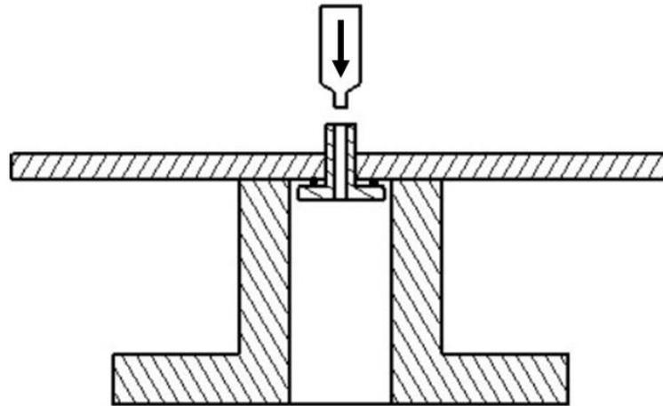
**Figure 5.** Testing procedure for destructive tensile rupture test.
