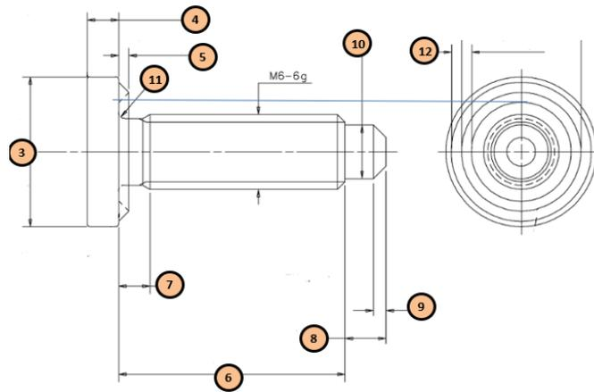
**Figure 3.** Ring shaped stud welding bolt schematic
