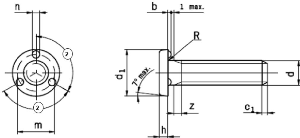
**Figure 1.** Triple projection weld stub/bolt
