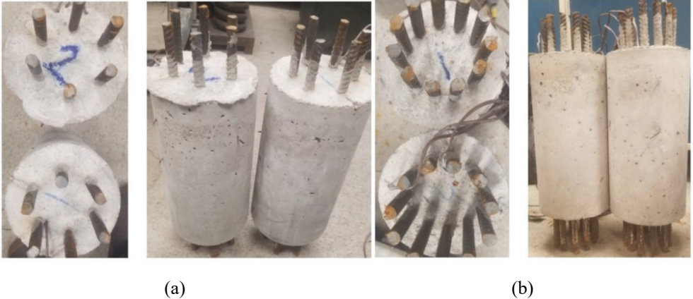
Figure 3 - Reinforced specimens (a) Mortar + 6 steel rebars (b) Mortar + 11 steel rebars
