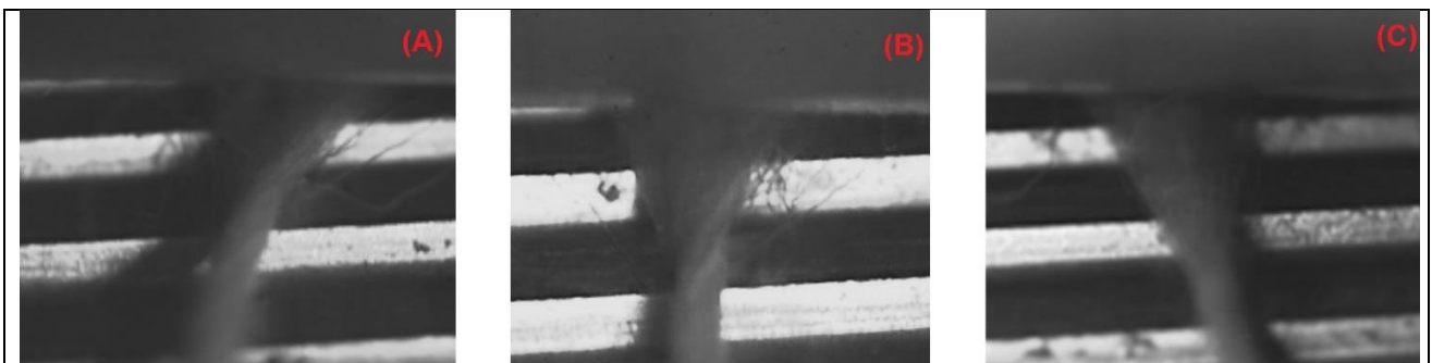
Şekil 3. Sol (A), normal (B) ve sağ (C) diyagonal eğirme düzeni (Left (A), normal (B) and right (C) diagonal spinning arrangement) (Wu vd., 2011)
