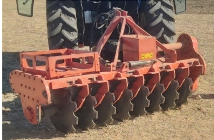
Figure 1. PTO driven the single-acting disc harrow used in the trials
