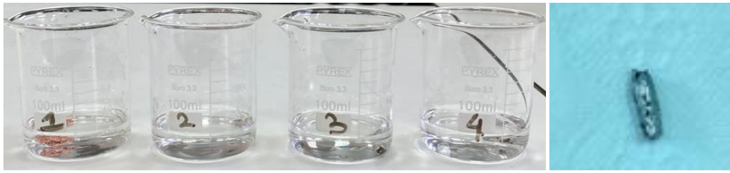
Figure 2. Soldered samples in 20%NaOH corrosion test solution
