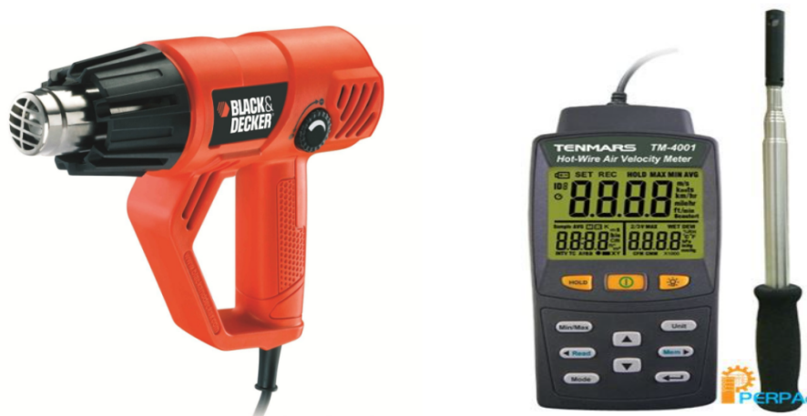
Figure 2.4 The view of the air guns used in the experiments and the anemometer reading the air velocity values.
