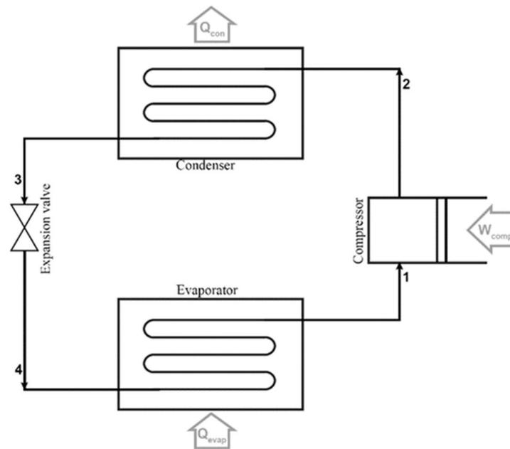
**Figure 2.** Schematic illustration of the vapor-compression refrigeration cycle
