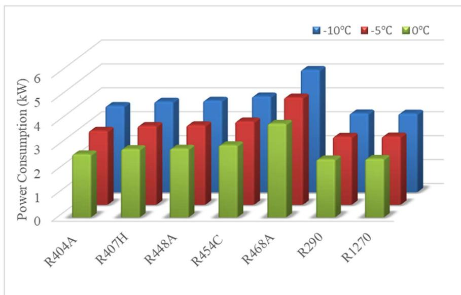
**Figure 4.** Power consumption of R404A and its alternatives
