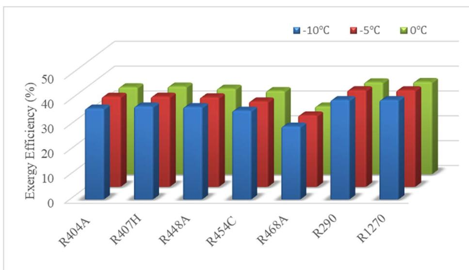
**Figure 6.** Exergy efficiency of R404A and its alternatives
