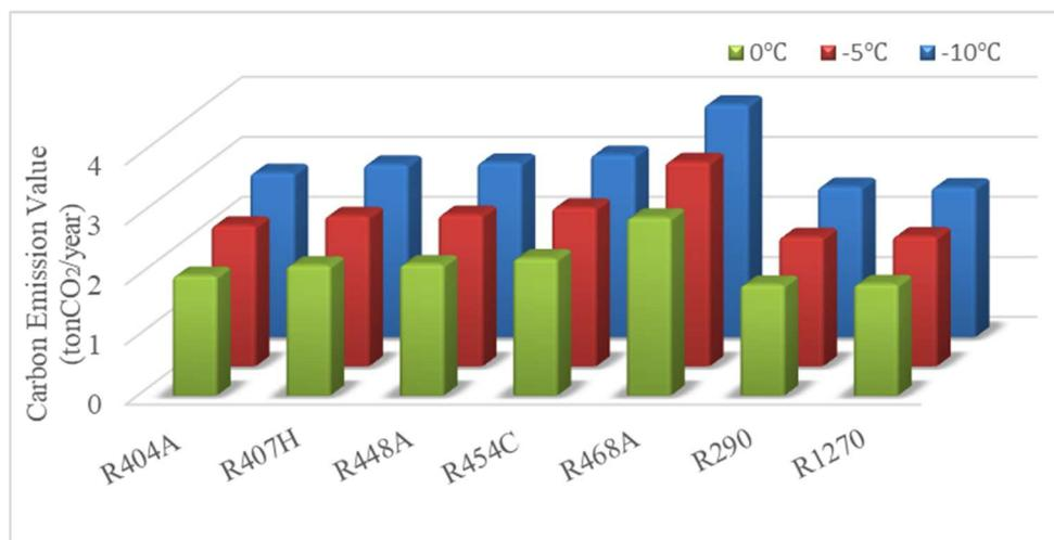
**Figure 7.** Annual total CO<sub>2</sub> emissions for R404A and its alternatives
