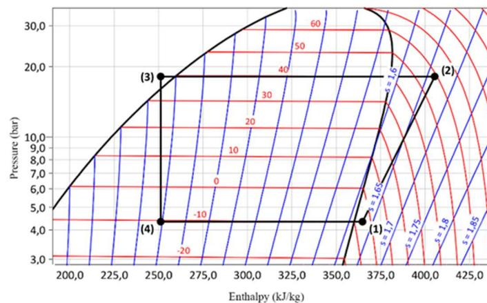
**Figure 3.** Log P - h diagram of R404A refrigerant
