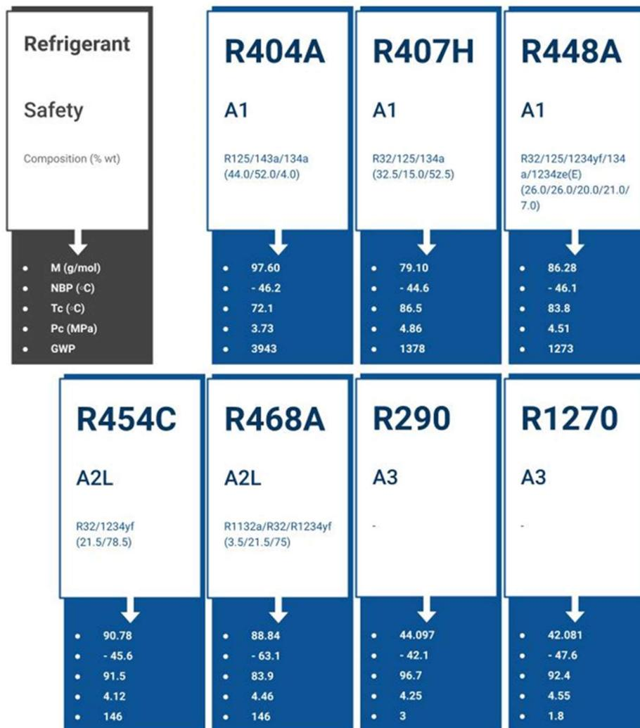
**Figure 1.** Chart of the characteristics of R404A and its alternative refrigerants
