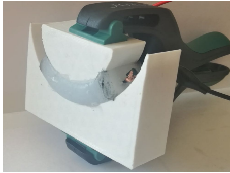
Figure 5. The test specimen was placed and clamped on the bending test setup.
