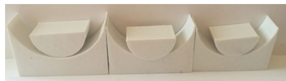
Figure 4. 3D printed bending test apparatus.
