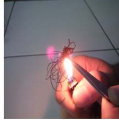
Figure A. The tensile strength values for the 250°C sample (1); flammability test of thermal stabilization sample at 250°C (2)
