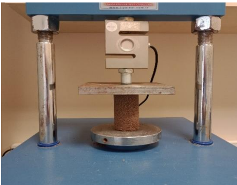
Figure 5. A photo from the uniaxial compressive strength test
