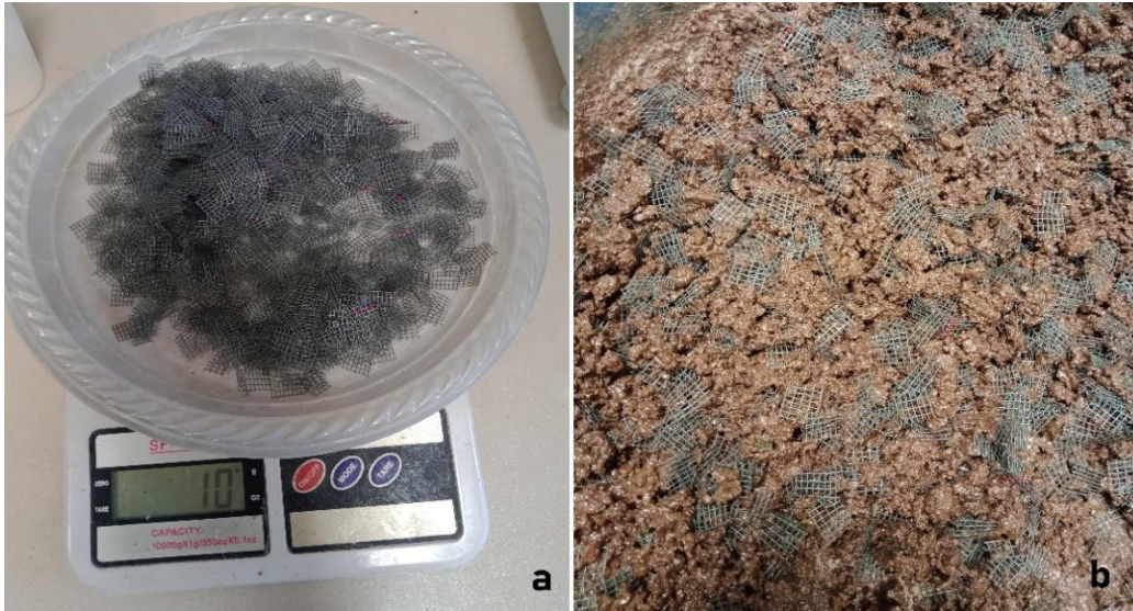
Figure 2. a) A photo from weighing processes, b) a view of MGF added soil mix
