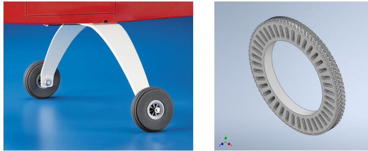
Figure 1. A sample of a basic drone landing gear with wheels (on the left) (Anonymous, 2023a) and an airless wheel modeled in Autodesk Inventor Pro
