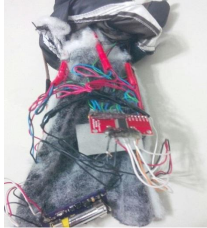
Figure 1: Parts of the glove [Upper part of the glove (16-Channel Analog/Digital Multiplexer and AAA battery unit)]
