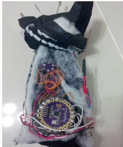
Figure 2: Parts of the glove [Lower part of the glove (Lilyaped, ADXL335, Flex and force sensors)]
