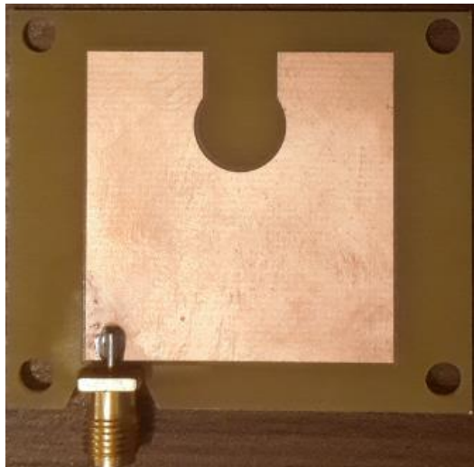
(b): Top view of the fabricated antenna.
