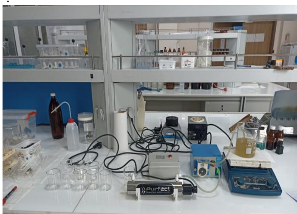
Figure 2. The experimental setup used in the feasibility study of treating with the UV/H 2 O 2 process
