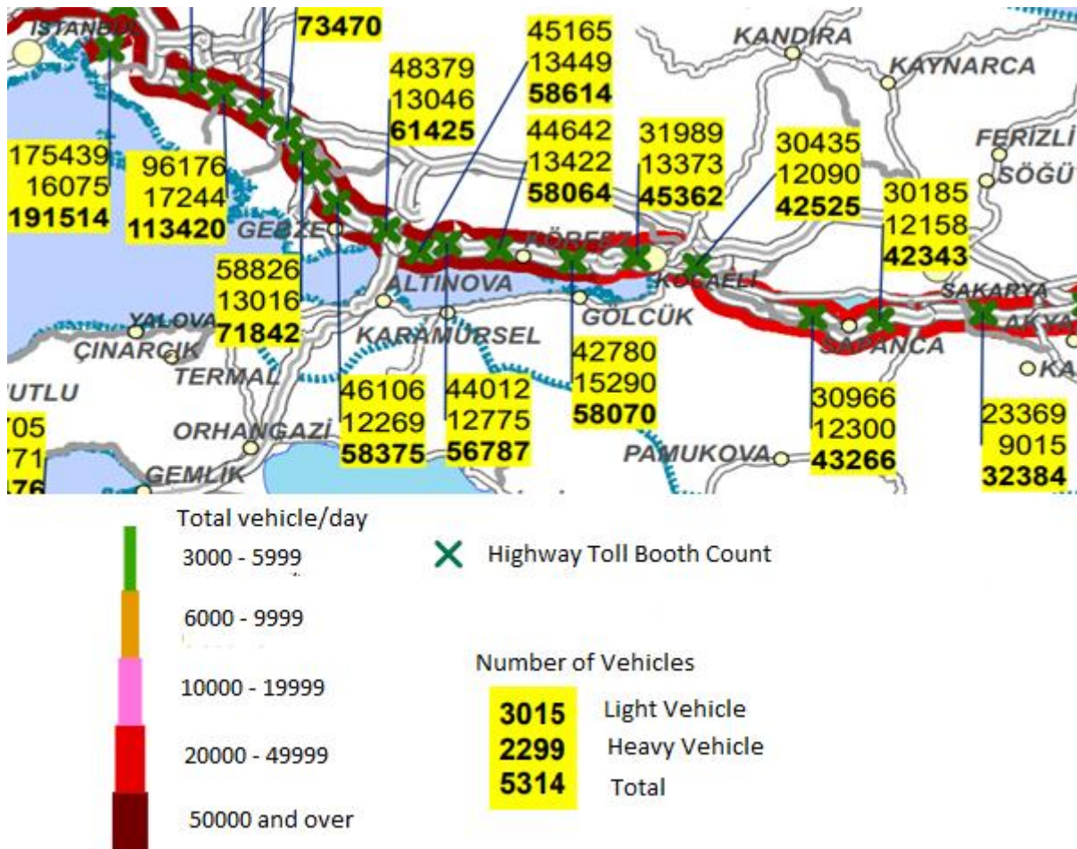
Figure 2. Highway Traffic Volume Map (2022), Annual Average Daily Traffic Value (Developed by the author using Karayolları Genel Müdürlüğü Traffic Volume Maps)
