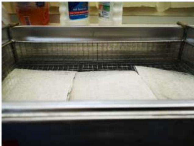
Figure 5. Washing of the carpets in the ultrasonic tank
