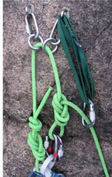
Figure 6. Lowering – End-Feed Method: For simplicity, the personal anchoring system (PAS) is omitted in the photograph. The green sling to the right represents either a quick draw for leaders, or a top-rope setup. A Figure Eight is tied and clipped to the harness. The original harness tie-in is removed, the end is fed through the anchor and it is then retied to the harness.
