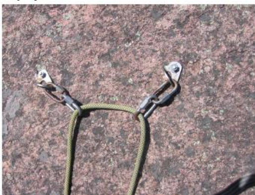
Figure 3. Expansion bolts with paired quick links.
