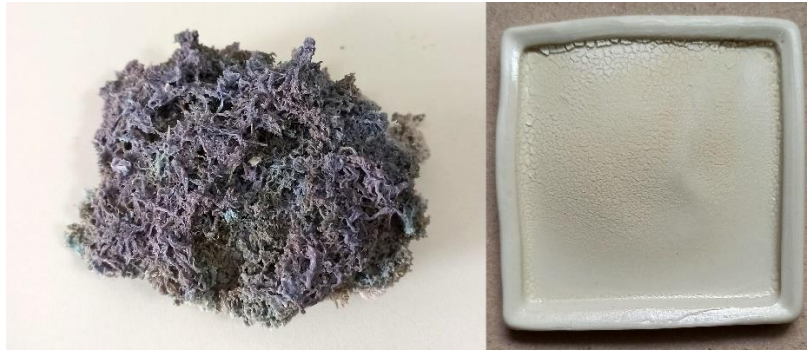
Figure 2a. Image of ash after calcination at 1000°C 2b. Image of calcined ash fired at 1200°C on porcelain plate.
