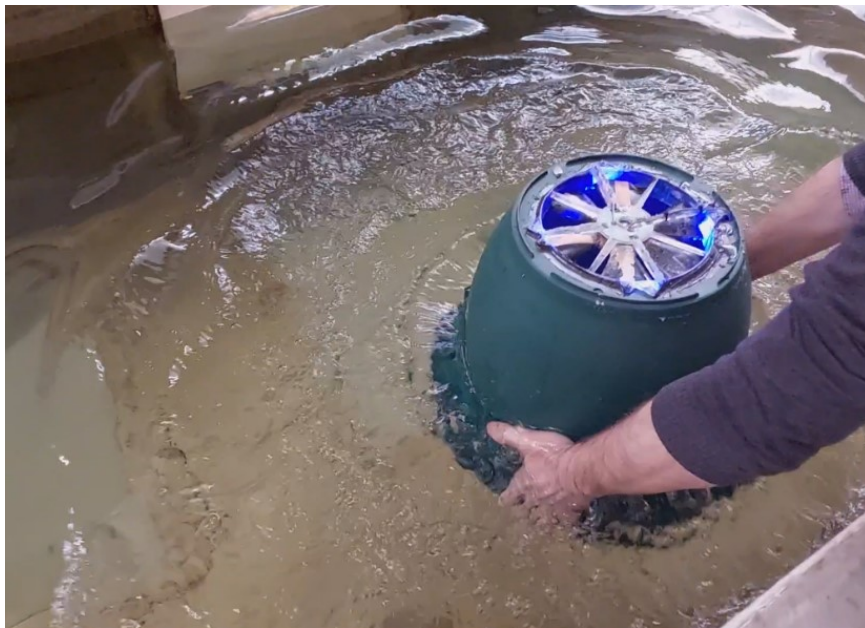
Figure 10. Four 3.4 V blue LEDs are illuminated.
