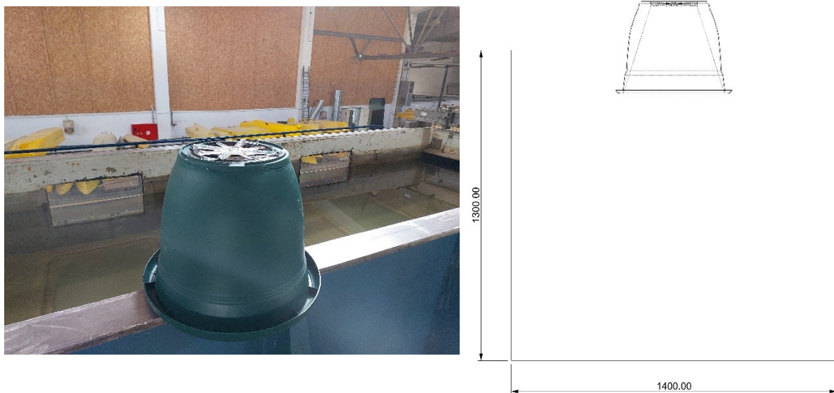
Figure 9. The OWC model and schematic layout of the model and the tank geometry.
