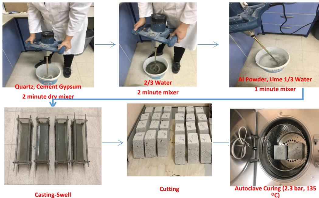
Figure 4. AAC production steps. included: a unit weight test, TS EN 772-13 and TS EN 771-4; a porosity test TS EN 772-4; a water absorption test TS
