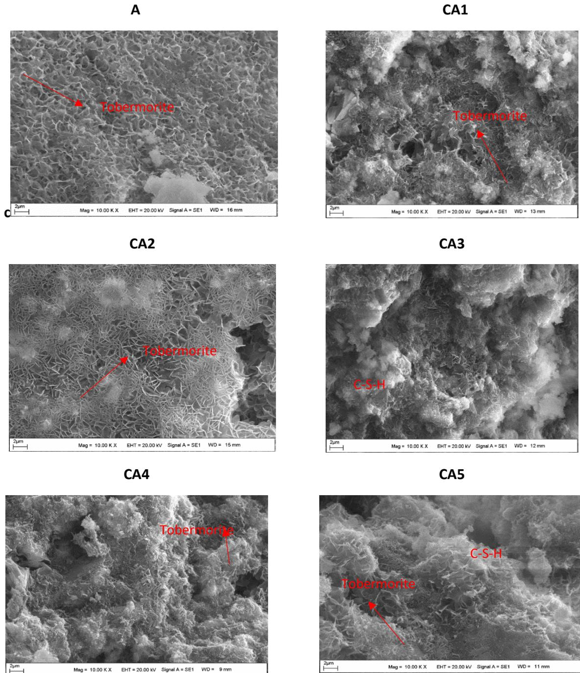
Figure 7. SEM images with glass waste AAC
