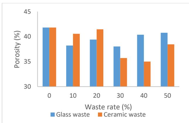
Figure 10. The porosity of AAC samples.
