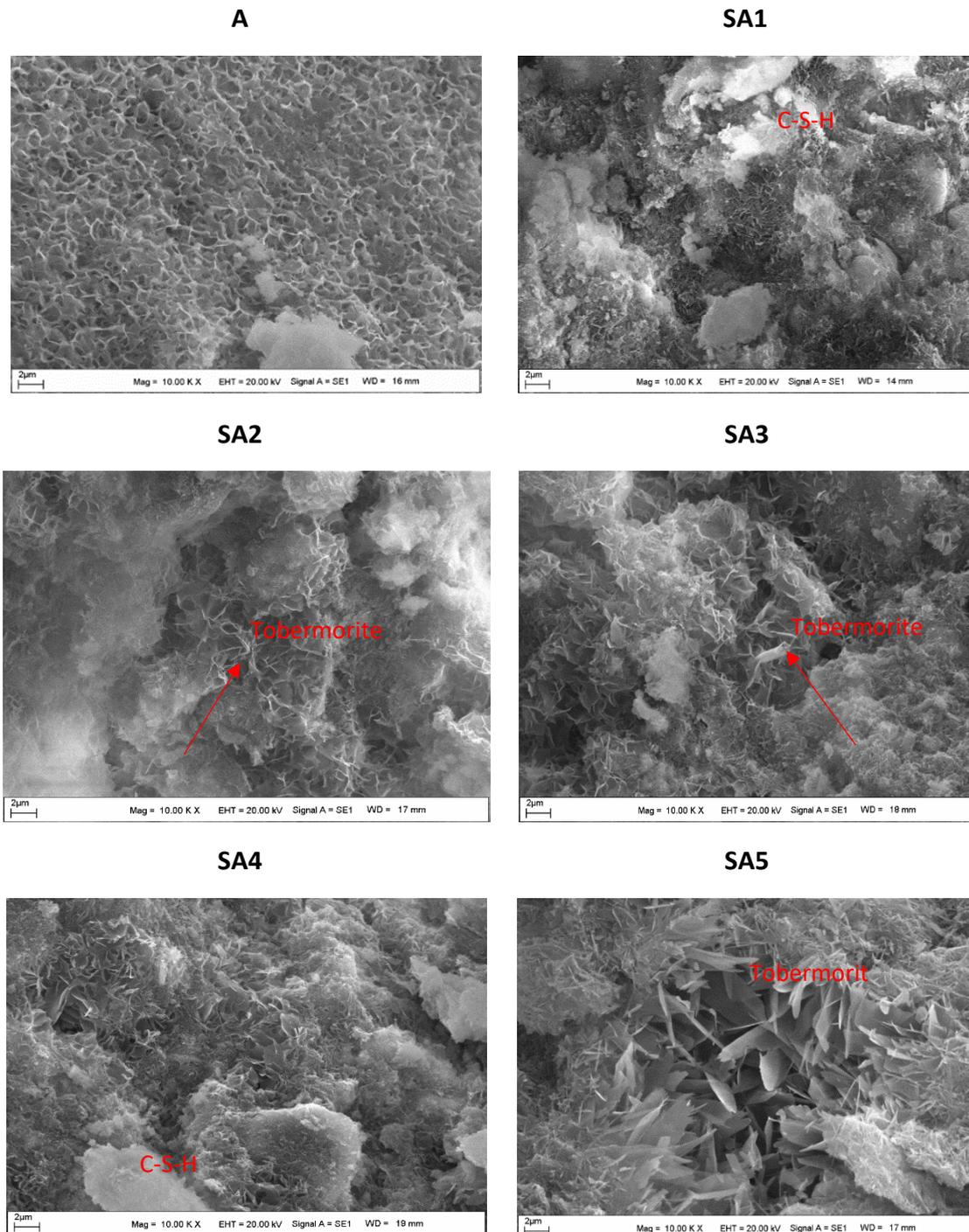
Figure 8. SEM images with ceramic waste AAC
