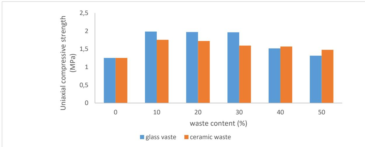
Figure 12. Uniaxial compressive strength of AAC samples.
