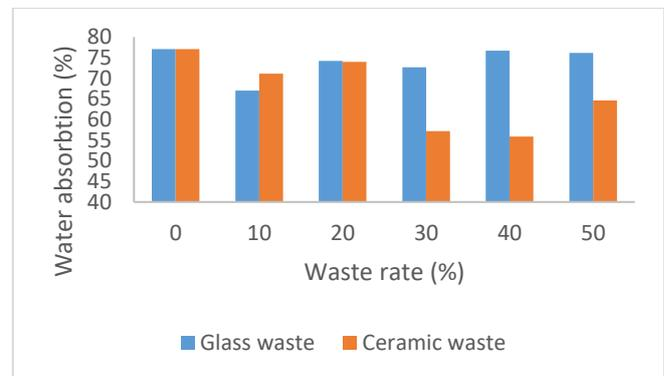
Figure 11. Water absorption values of AAC samples.
